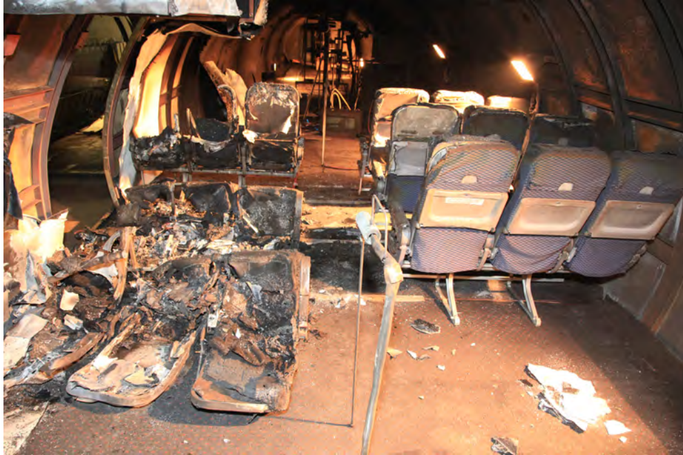
Figure 134. The WE-43 Repeat Test With Additional Magnesium Alloy Components, Aft View
