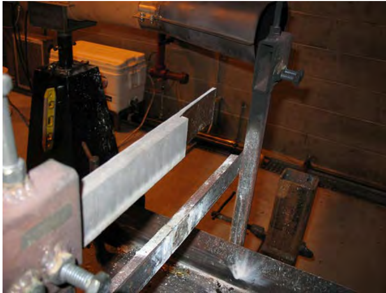
Figure 27. Sectioned Bar Sample Positioned Horizontally in Front of the Burner
