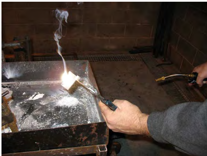
Figure 24. Thin Sliver of Magnesium Alloy on Fire After Being Heated With Torch
