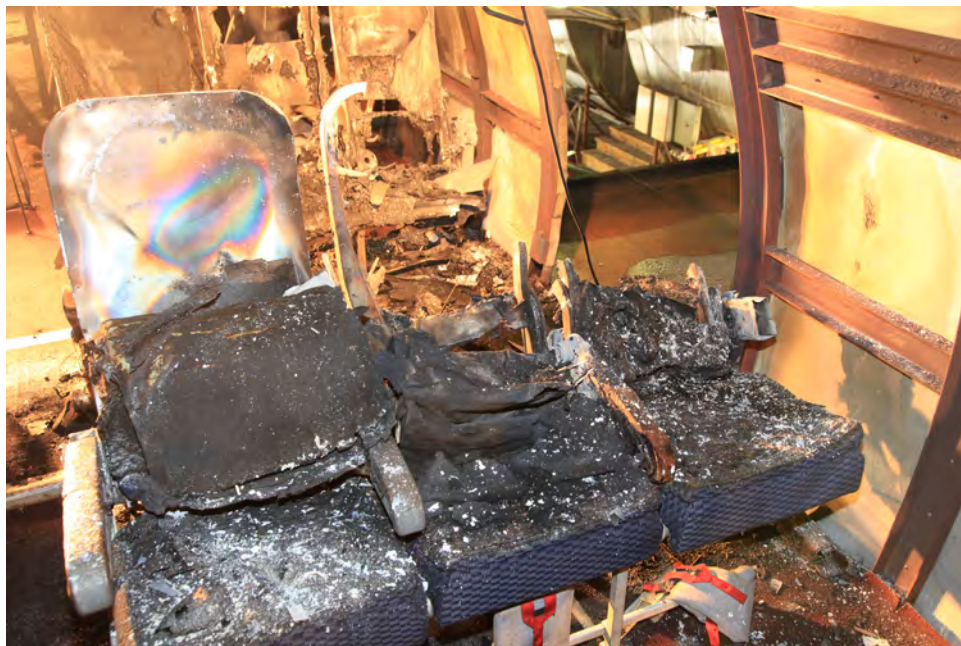
Figure 108. Portside Row 1 Seat Assembly Posttest for the AZ-31 Magnesium Alloy Test
