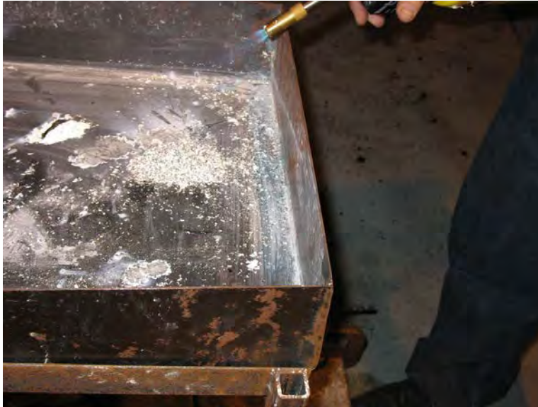
Figure 21. Torch Used to Ignite a Small Pile of Magnesium Alloy Millings
