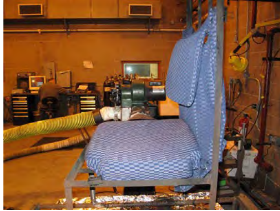
Figure B-20. Side View of Baseline Test 2 Cushions Prepared for Testing in Laboratory-Scale Test Rig
