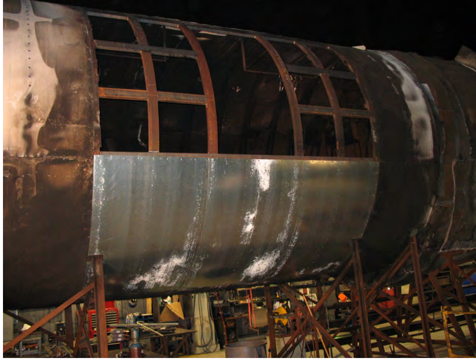
Figure 30. Construction of Steel Test Fuselage Showing Curved Steel Channels
