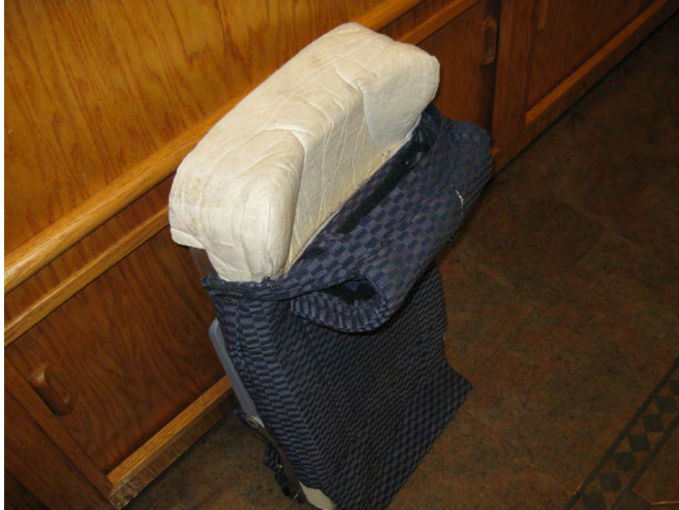
Figure 72. Dress Cover Being Test Fitted to Prototype Cushion Assembly
