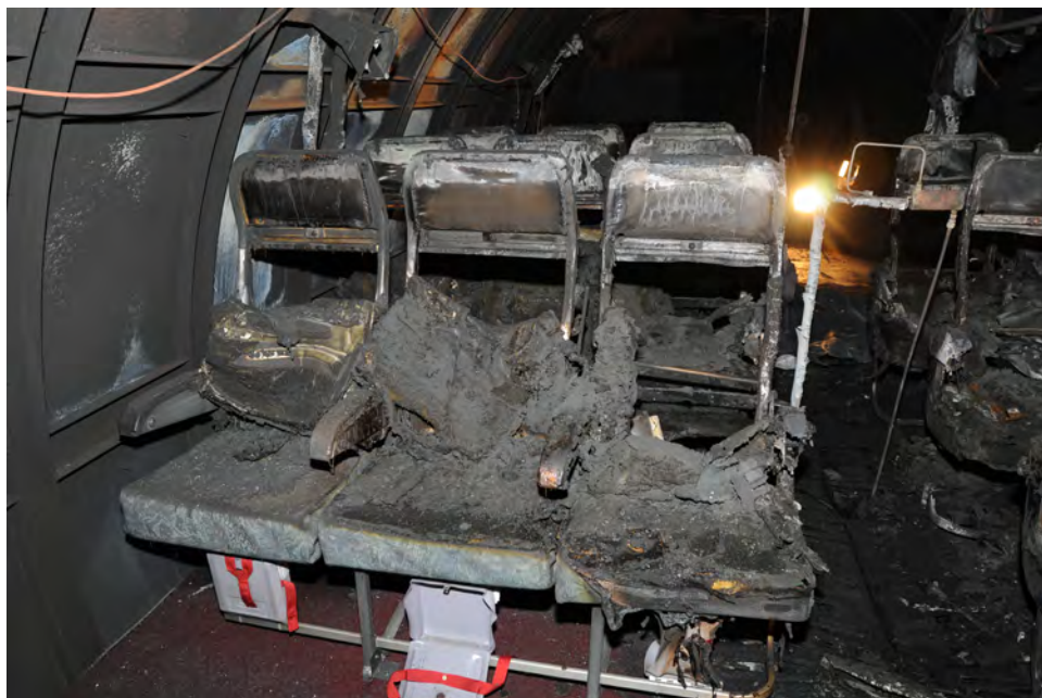
Figure 43. Seatback Materials Consumed and Cushioning Remnants Displaced
