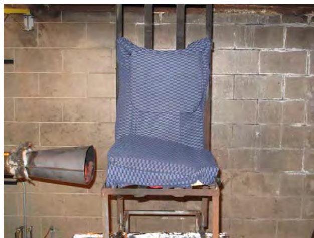
Figure B-19. Front View of Baseline Test 2 Cushions Prepared for Testing in Laboratory-Scale Test Rig
