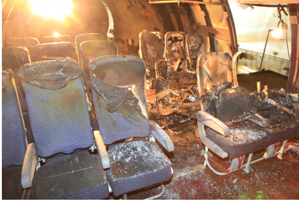
Figure 107. Posttest Conditions for AZ-31 Magnesium Alloy
