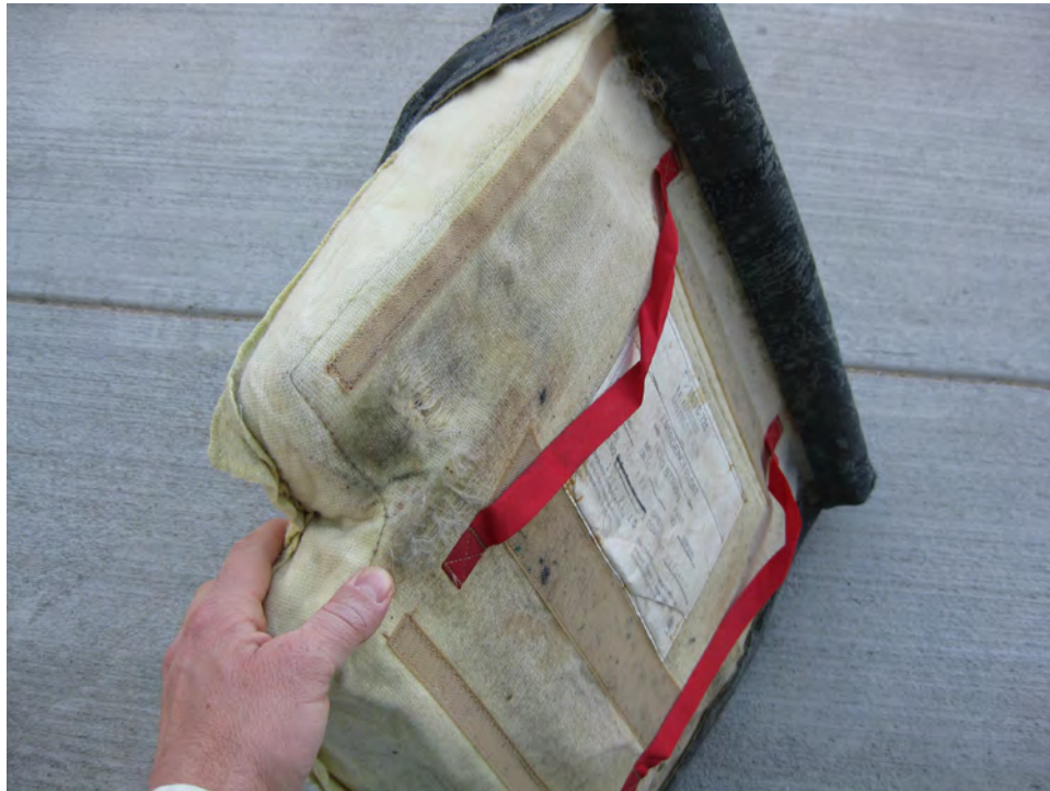
Figure B-5. Side View of Baseline Test 1 Bottom Seat Cushion With B/E Aerospace Fire-Blocking Layer
