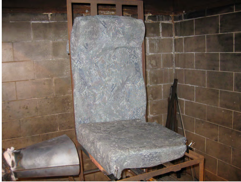
Figure B-11. Baseline Test 1 Cushions Attached to Laboratory-Scale Test Rig
