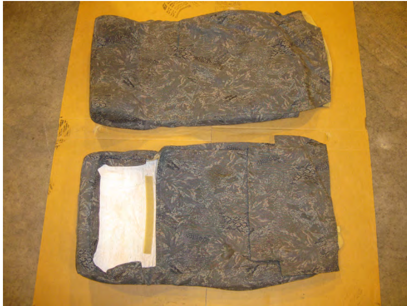
Figure B-10. Baseline Test 1 Back Cushion Containing Fiberfill Material
