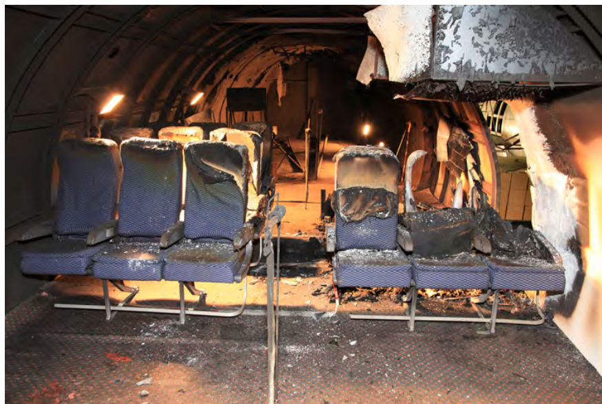
Figure 133. The WE-43 Repeat Test With Additional Magnesium Alloy Components, Posttest
