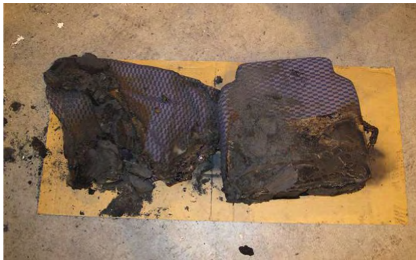
Figure B-23. Baseline Test 2 Cushion Samples Following Laboratory-Scale Test
