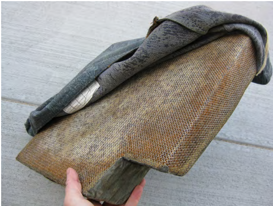
Figure B-3. Baseline Test 1 Bottom Seat Cushion (style 1) Revealing No Fire-Blocking Layer
