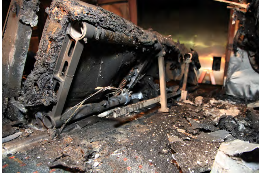
Figure 136. The WE-43 Repeat Test With Additional Magnesium Alloy Components, Close-Up of Portside Row 2 Seat Structure
