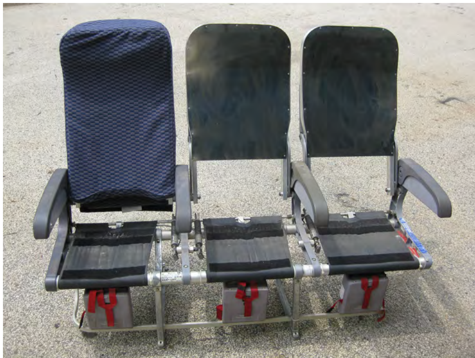
Figure 74. Partially Fabricated Seatbacks Showing Front Aluminum Pan
