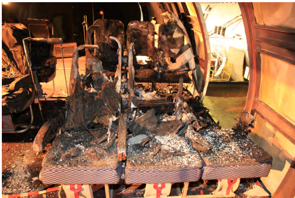
Figure 82. Close-Up of Portside Triple Seats Showing Melted Aluminum Seatbacks
