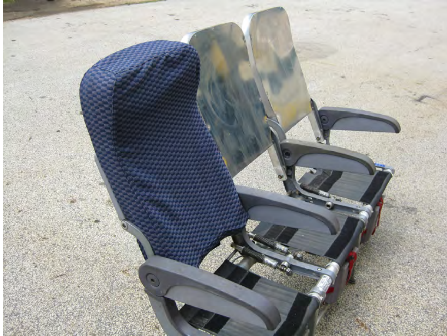
Figure A-7. Partially Completed Seat Assemblies Showing Front Pan Structure
