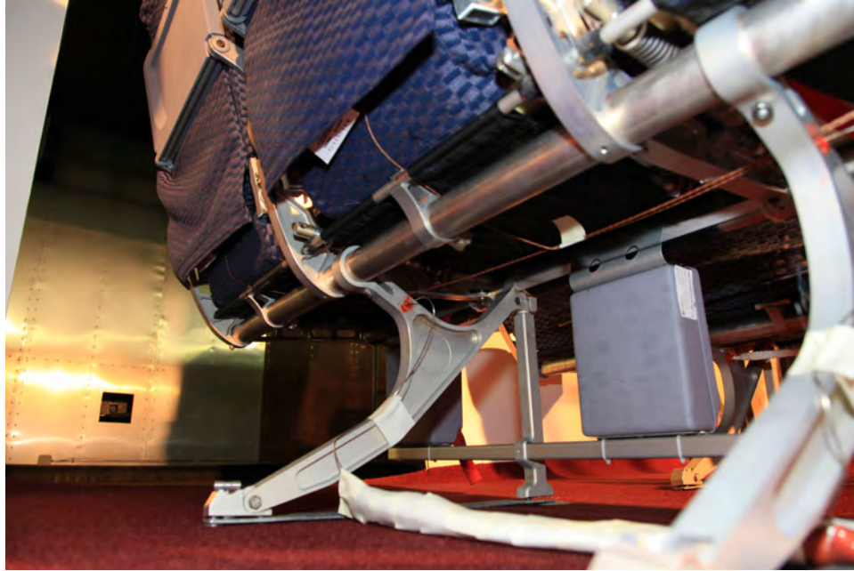
Figure 106. The AZ-31 Components Showing Thermocouple Installed on the Leg Component
