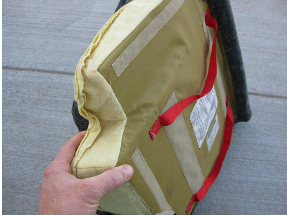
Figure B-8. Side View of Baseline Test 1 Bottom Seat Cushion With Franklin Products Fire-Blocking Layer
