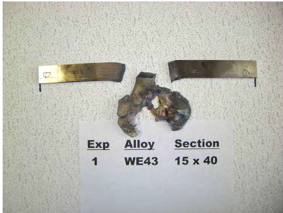
Figure 7. Posttest Inspection Showing Molten Center Section Removed From Catch Pan
