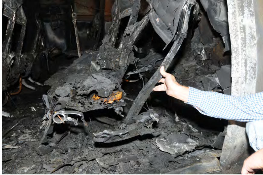
Figure 44. Portside Row 2 Seat Primary Spreader Component
