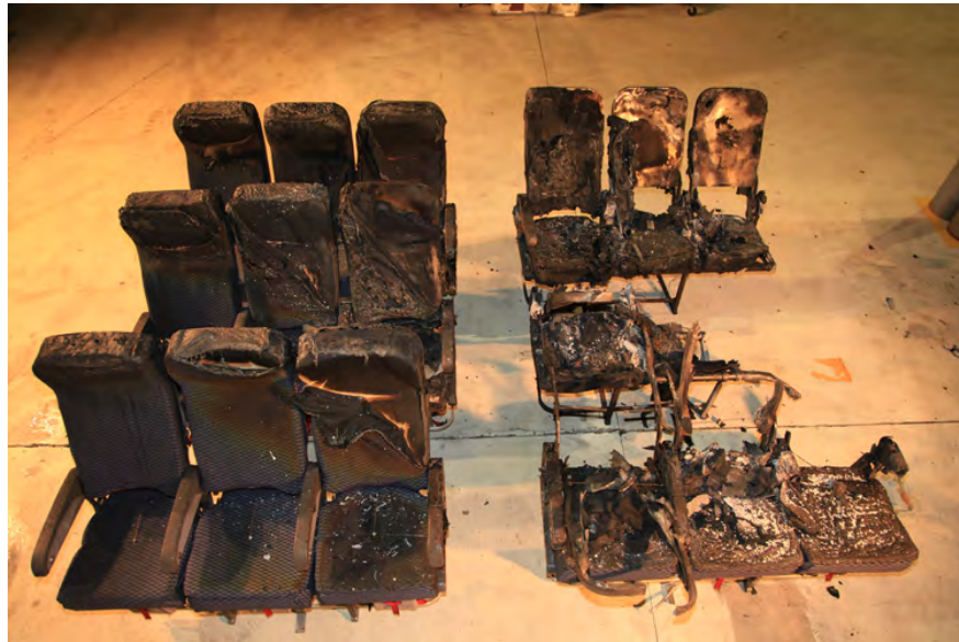
Figure 85. Seats Removed From Fuselage Following Baseline 3 Test
