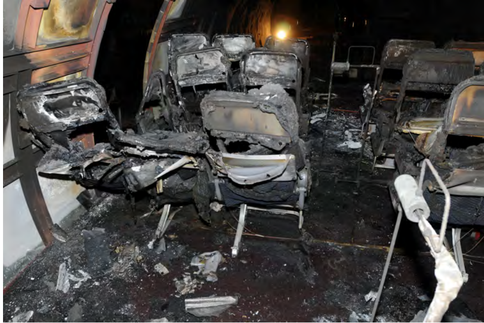
Figure 64. Aft Cabin View of Portside Seats Showing Back Assembly Structure Collapse
