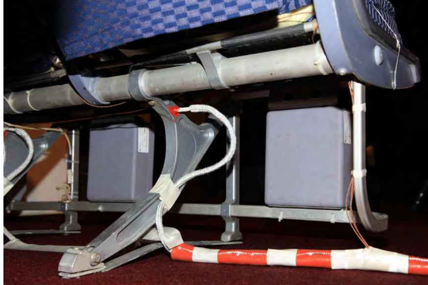
Figure 77. Typical Embedded Thermocouple Arrangement in Seat Leg
