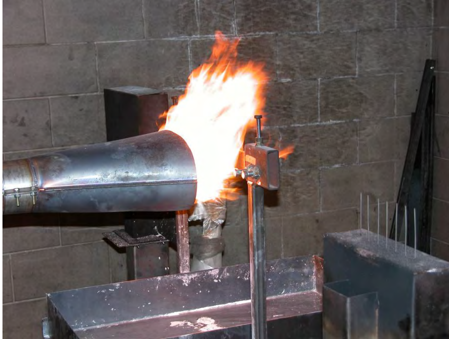
Figure 3. Magnesium Alloy Bar Sample Exposed to Burner Flames
