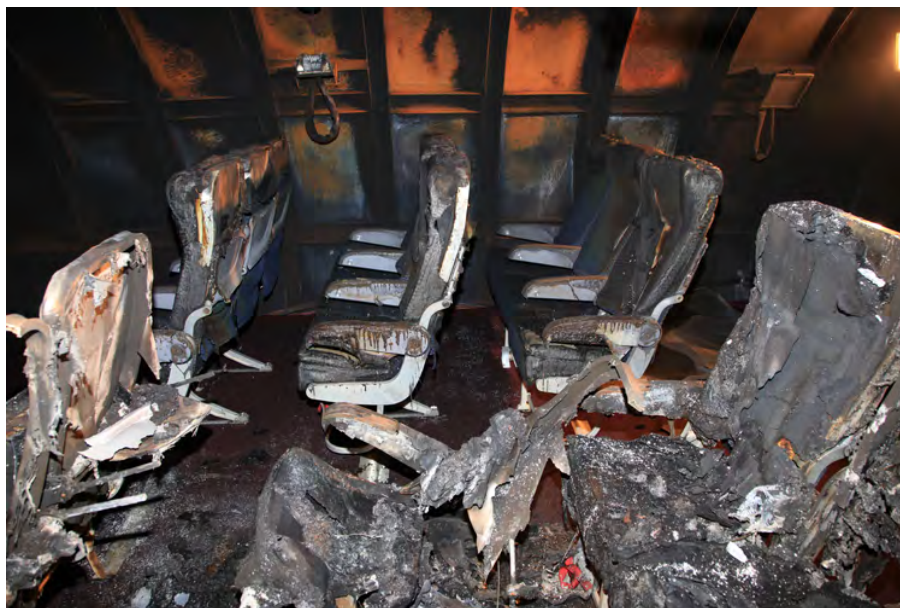
Figure 110. Portside Row 2 Seat Frame Damage Following AZ-31 Magnesium Alloy Test
