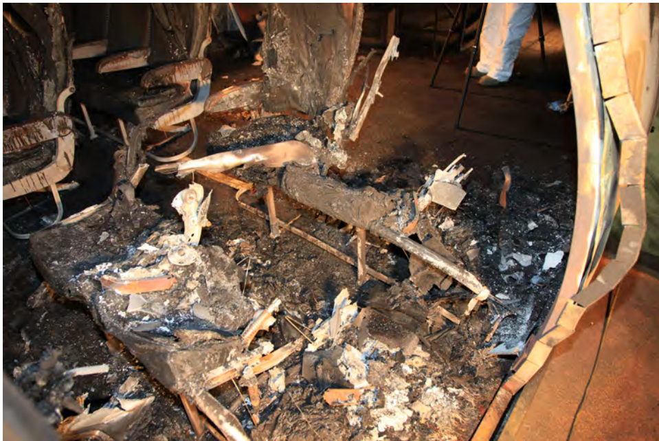
Figure 127. View of Row 2 and Row 3 Seat Assemblies Through Fire Opening
