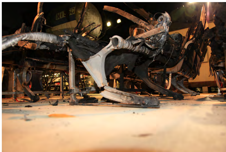
Figure 86. Close-Up of Melted Seat Structure Primary Components
