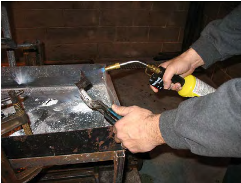
Figure 23. Thin Sliver of Magnesium Alloy Being Heated With Torch
