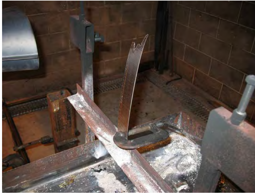
Figure 25. Longitudinal Slice of Magnesium Alloy Positioned Vertically in Front of the Burner
