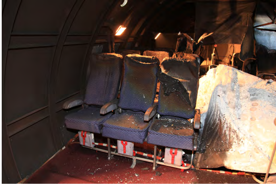
Figure 83. Posttest Starboard-Side Seats in Baseline Test 3
