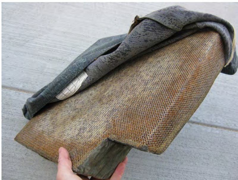
Figure 56. Side Angle View of Bottom Seat Cushion Used in Baseline Test 1 With no Fire-Blocking Layer or Inspection Tag
