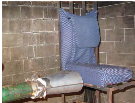
Figure B-22. Side View of Baseline Test 2 Cushions Prepared for Testing in Laboratory-Scale Test Rig
