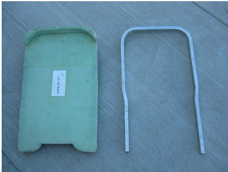
Figure 71. Fire-Hardened Foam and Fabricated Aluminum Frame
