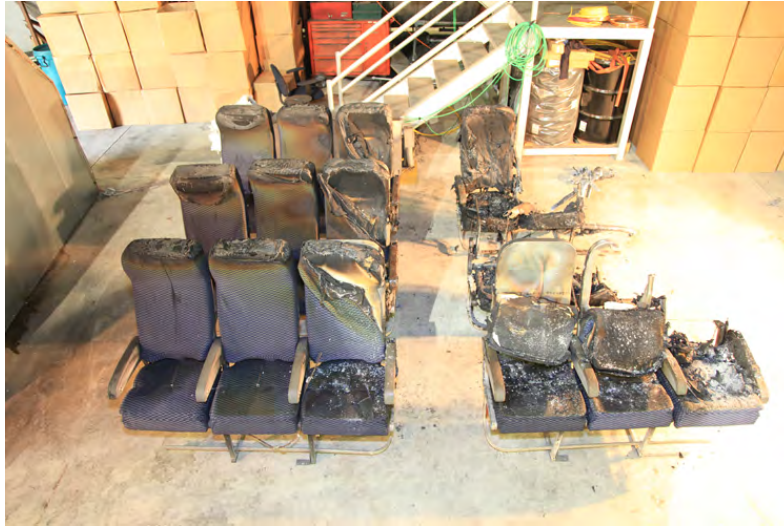
Figure 130. The WE-43 Test With Additional Magnesium Alloy Components, Seats Placed on the Test Facility Floor
