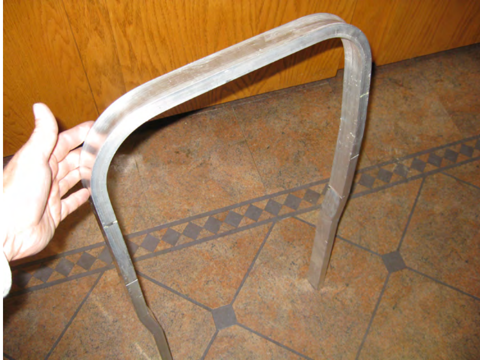
Figure A-2. Aluminum Seatframe Used in Alternate Seatback Assembly
