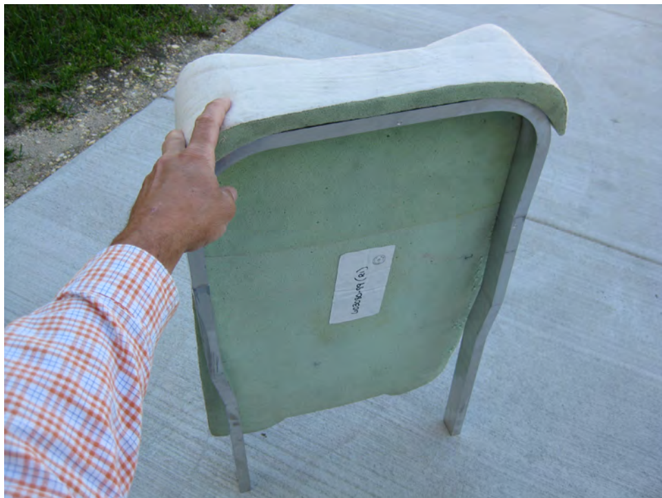
Figure A-3. Fire-Hardened Foam Used in Alternate Seatback Assembly
