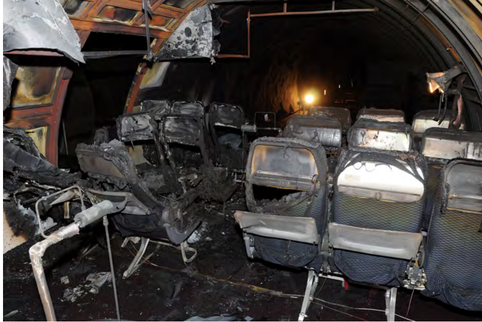
Figure 63. Aft Cabin View, Showing Portside and Starboard Seat Damage
