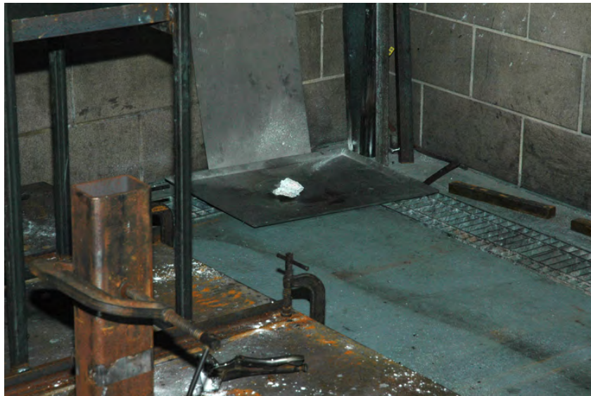
Figure 14. Molten Mass of ZE-10 Alloy Removed From the Catch Pan and Placed on the Floor
