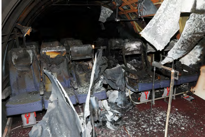
Figure 60. Baseline Test 2 Cabin Materials Following Test Fire
