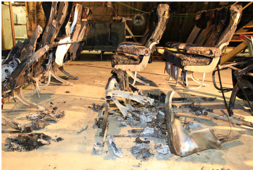
Figure 104. Seat Frames on the Floor of the Test Facility Showing Evidence of Magnesium Burning
