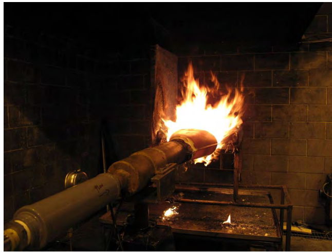
Figure A-8. Baseline Test 3 Cushion Sample During Laboratory Test (typical)
