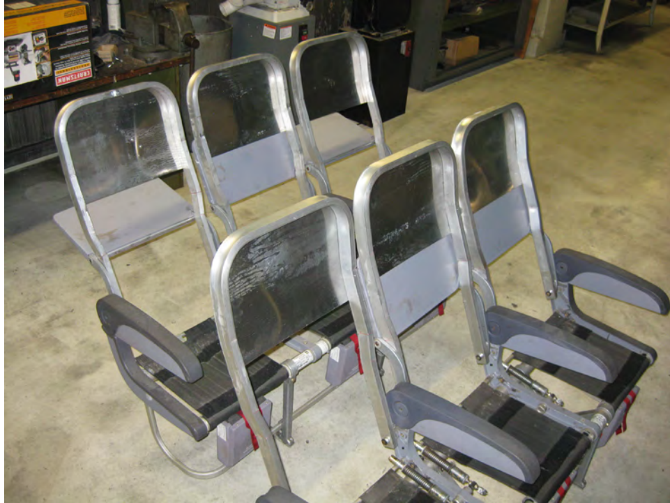
Figure 73. Seatback Assemblies Being Fabricated and Mounted on B/E 990 Seats
