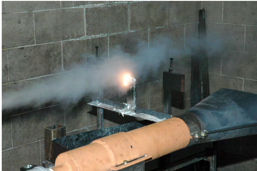
Figure 12. Extinguisher Stream Being Directed Across Burning Magnesium Alloy Sample
