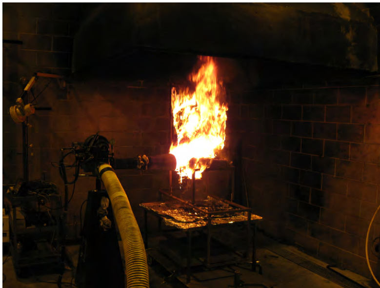
Figure B-14. Baseline Test 1 Bottom Seat Cushion During Laboratory-Scale Test (typical), Third Frame
