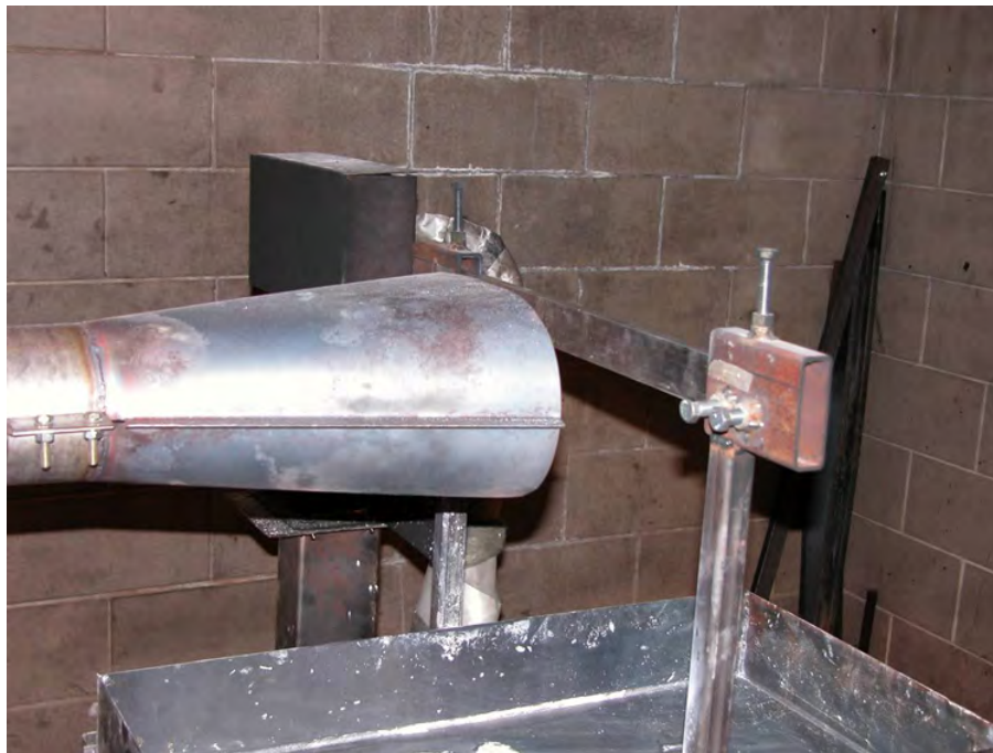
Figure 2. Magnesium Alloy Bar Sample Mounted in Test Apparatus Prior to Test
