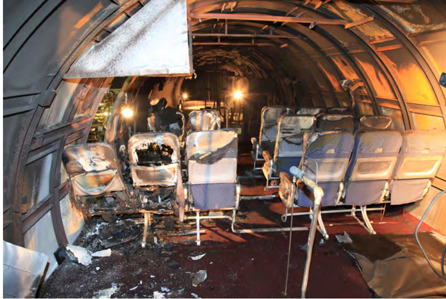
Figure 109. Aft View of Fire Damage for AZ-31 Magnesium Alloy Test
