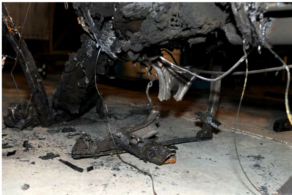
Figure 66. Close-Up View of Melted Leg and Cross Tube Structure on Entry Door Seat
