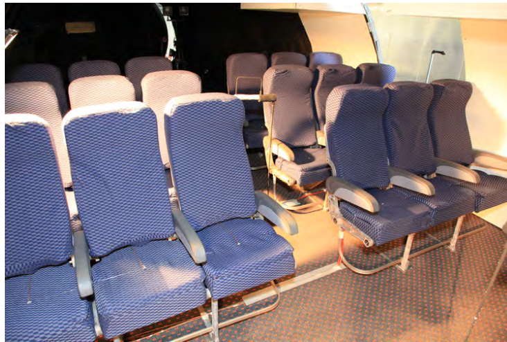
Figure 121. The WE-43 Test Configuration With Additional Magnesium Alloy Components
