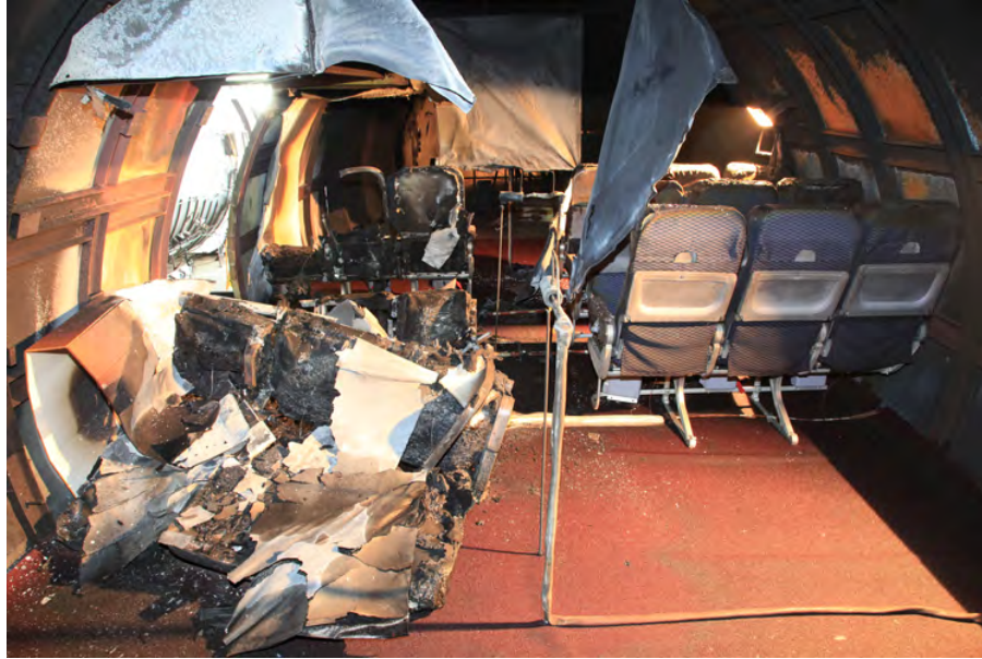
Figure 101. The WE-43 Magnesium Alloy Test Showing Portside Row 3 Seat Tipped Over
