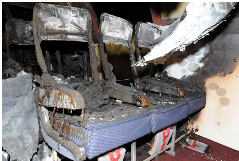
Figure 61. Close-Up View of Portside Triple Seat in the Baseline 2 Test
