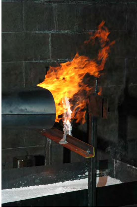
Figure 11. Vertically Mounted Sample Just Prior to Extinguisher Discharge
