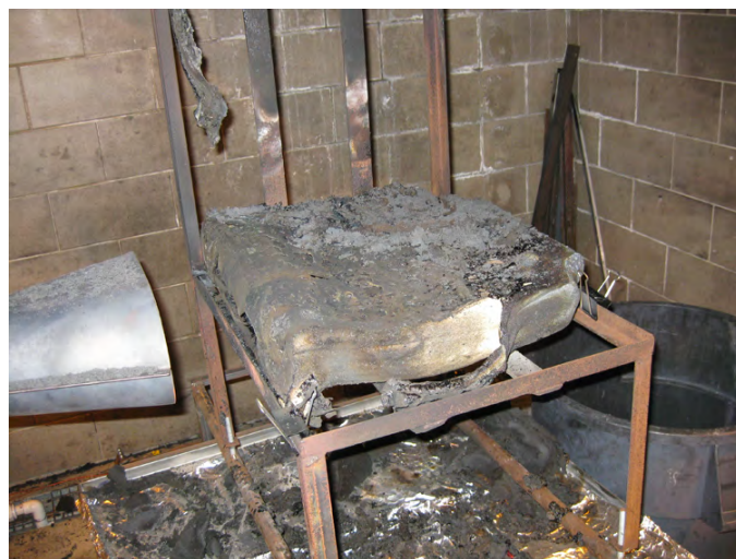
Figure B-16. Baseline Test 1 Cushion Following Laboratory-Scale Test (typical)
