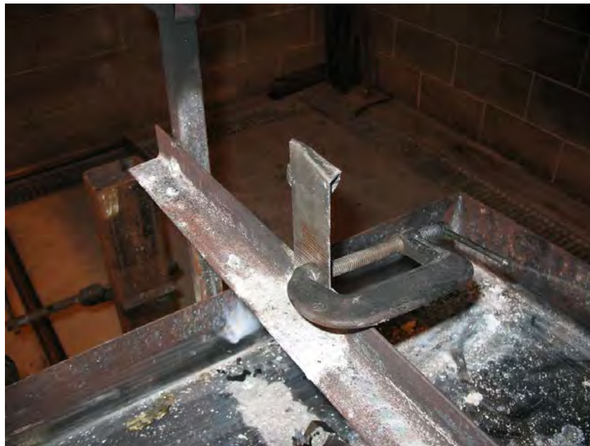
Figure 26. Vertically Mounted Slice After Self-Extinguishment
