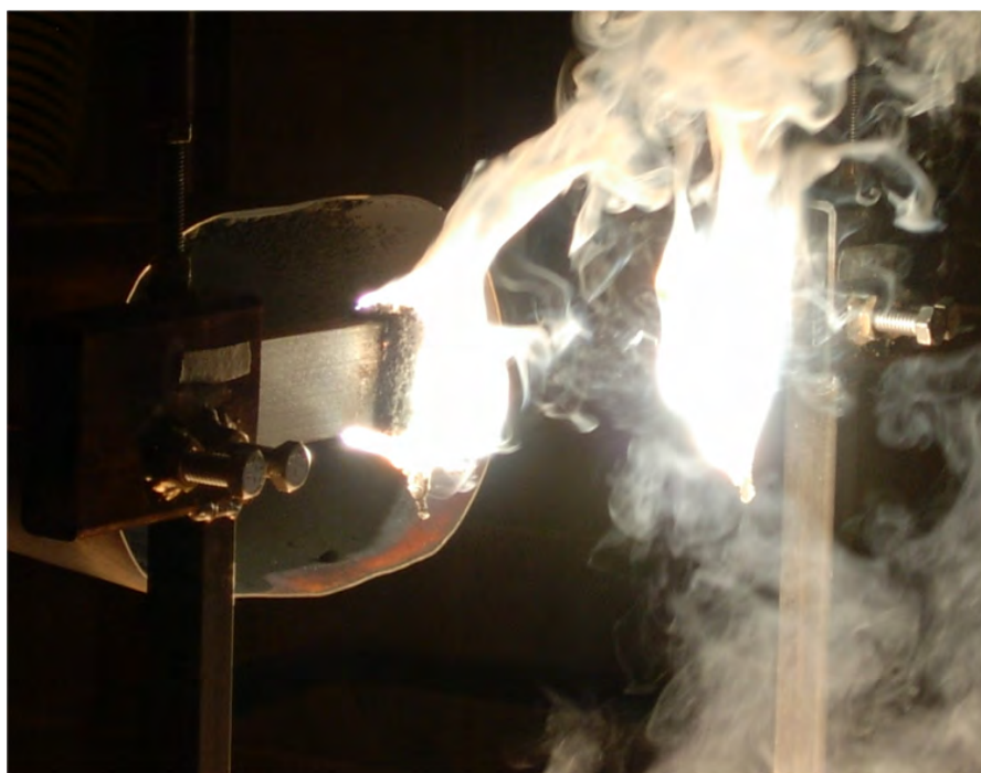
Figure 6. Ignition of Magnesium Alloy Following Burner Flame Exposure
