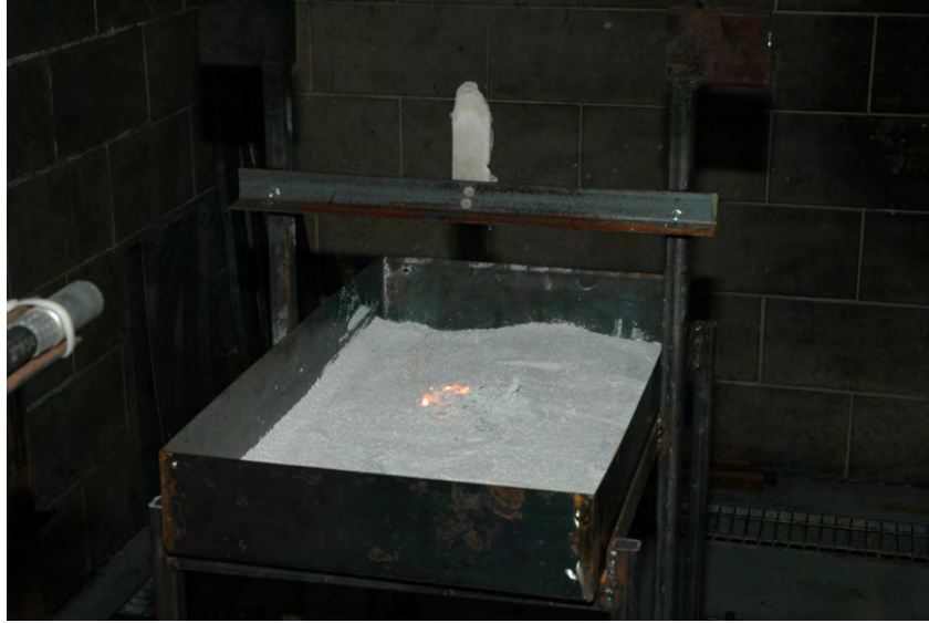
Figure 13. Section of Molten Test Sample in the Catch Pan After Extinguisher Discharge
