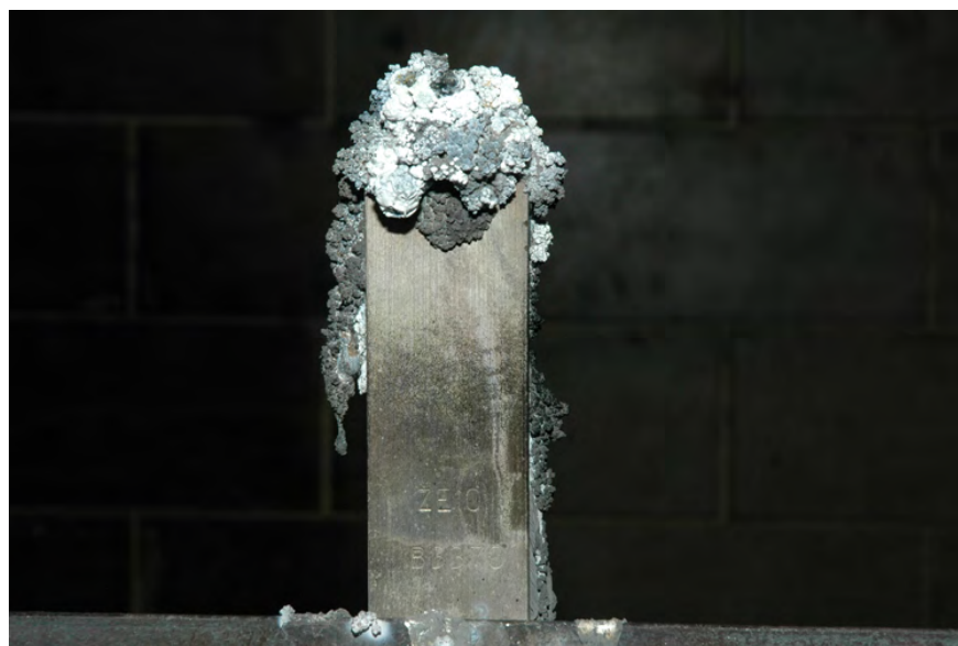
Figure 16. Strange Oxidation on ZE-10 Sample Following Agent Application
