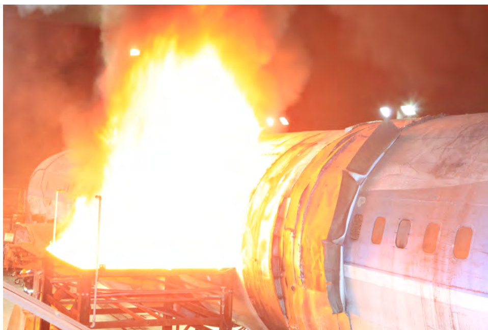
Figure 99. External Pan Fire During WE-43 Magnesium Alloy Test
