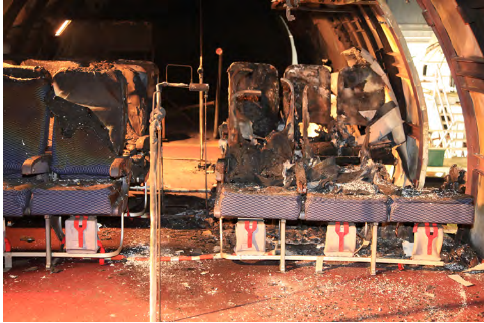
Figure 81. Baseline Test 3 Damage to Portside Seats
