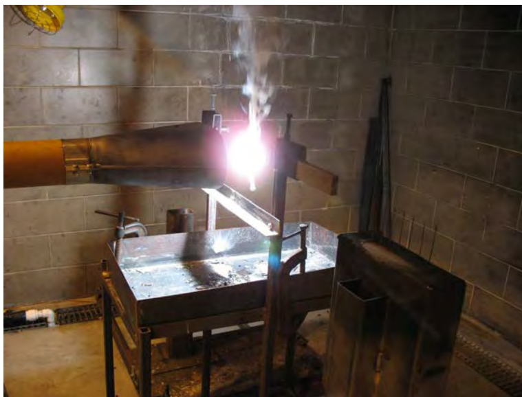
Figure 28. Sectioned Magnesium Alloy Bar Sample Ignited Using Oil Burner
