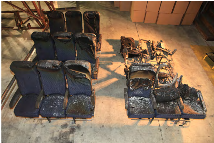
Figure 137. The WE-43 Repeat Test With Additional Magnesium Alloy Components, Seats on the Test Facility Floor
