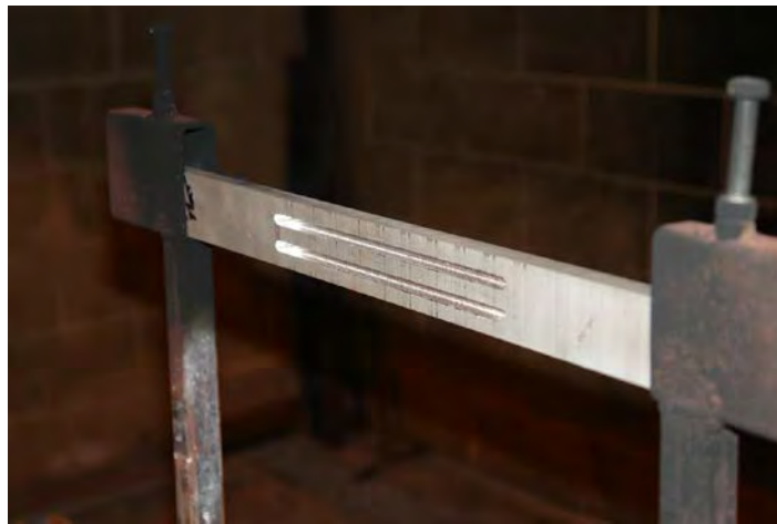
Figure 17. Magnesium Alloy Test Sample Bar With a Milled Cross Section
