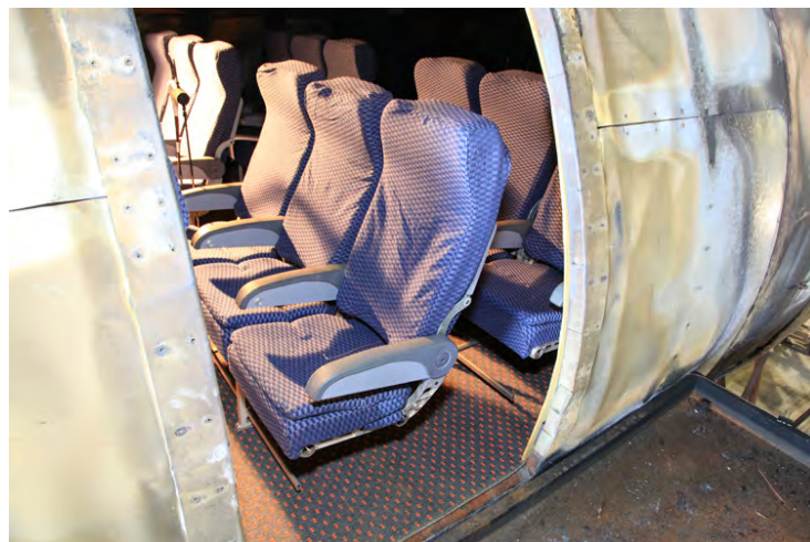
Figure 122. The WE-43 Test Configuration With Additional Magnesium Alloy Components Viewed Through the Fire Opening
