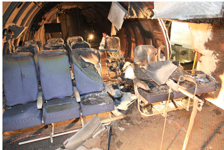
Figure 123. The WE-43 Test With Additional Magnesium Alloy Components, Posttest
