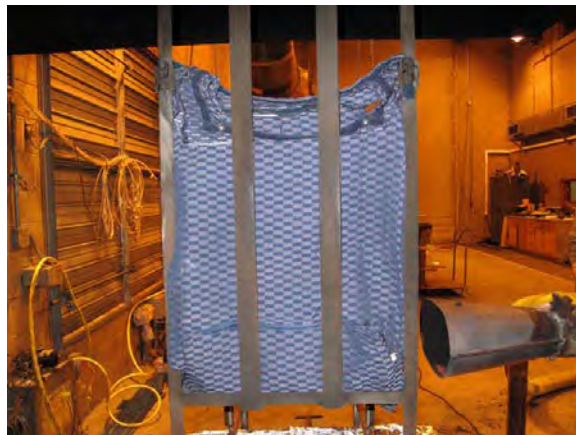
Figure B-21. Rear View of Baseline Test 2 Cushions Prepared for Testing in Laboratory-Scale Test Rig
