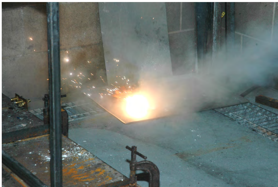
Figure 15. Molten ZE-10 Reacting to Stream of Halon 1211
