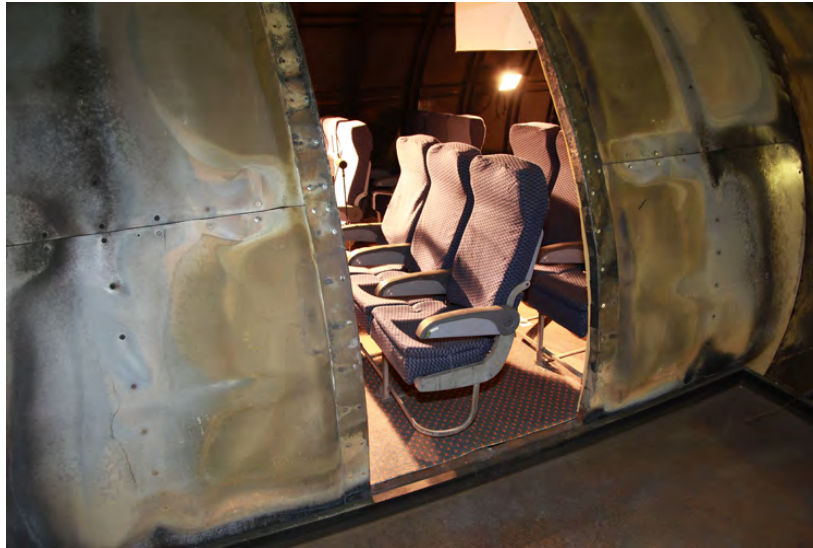
Figure 132. Starboard-Side Seat Assembly in Fire Opening, With Curved Baggage Bar (Repeat Test)
