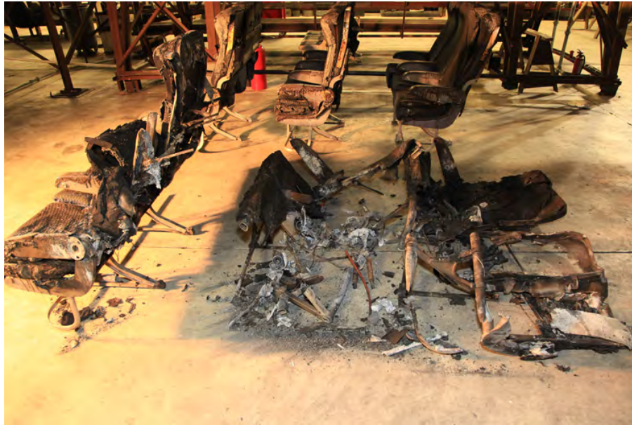
Figure 138. The WE-43 Repeat Test With Additional Magnesium Alloy Components, Damage to Portside Seat Assemblies
