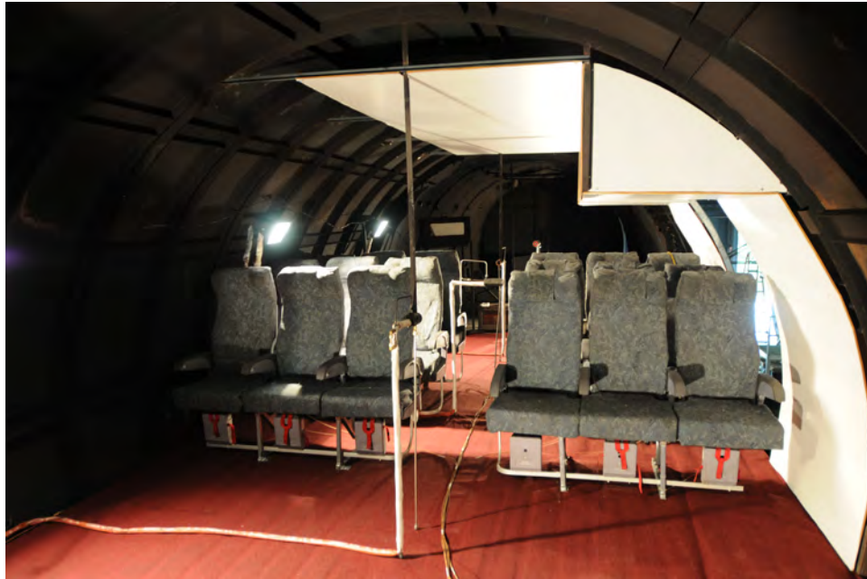
Figure 33. Typical Full-Scale Test Configuration With Seats, Panels, and Carpet Installed
