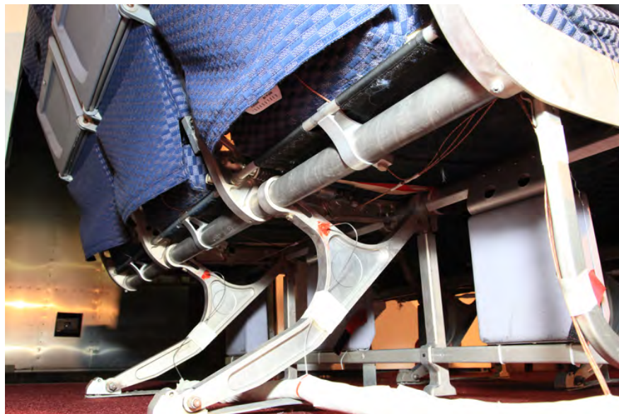
Figure 98. The WE-43 Primary Components With Thermocouples Embedded in the Legs
