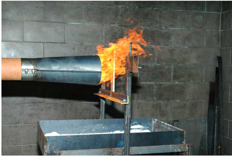
Figure 9. Magnesium Alloy Sample Mounted Vertically
