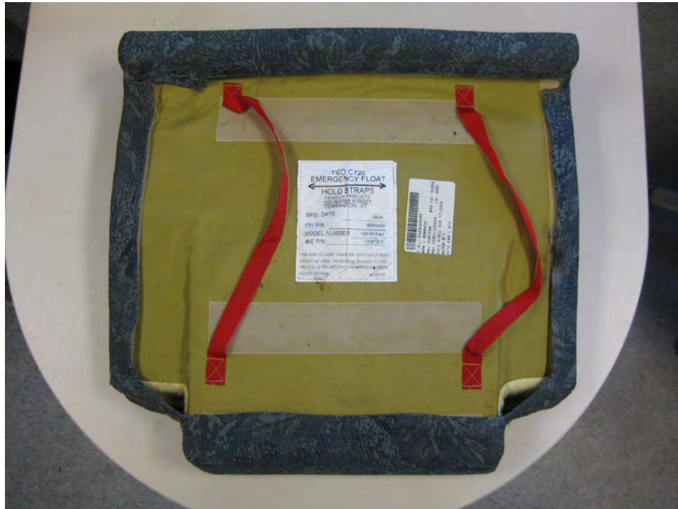
Figure B-7. Baseline Test 1 Bottom Seat Cushion With Franklin Products Fire-Blocking Layer
