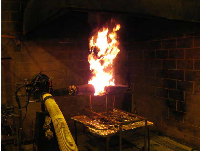
Figure B-13. Baseline Test 1 Bottom Seat Cushion During Laboratory-Scale Test (typical), Second Frame
