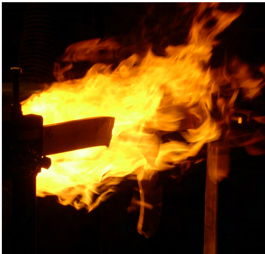
Figure 5. Center Section of Bar Sample Falling Into Catch Pan After Melting
