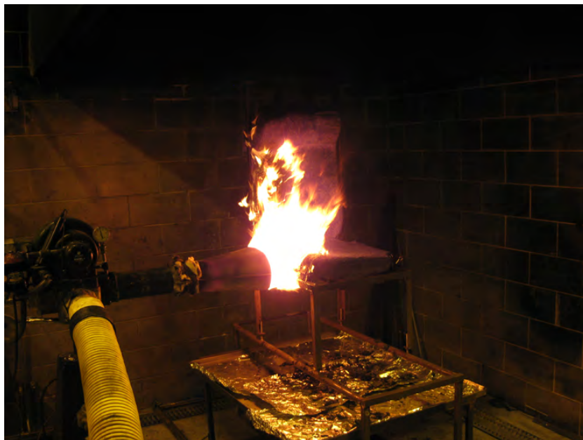
Figure B-12. Baseline Test 1 Bottom Seat Cushion During Laboratory-Scale Test (typical), First Frame
