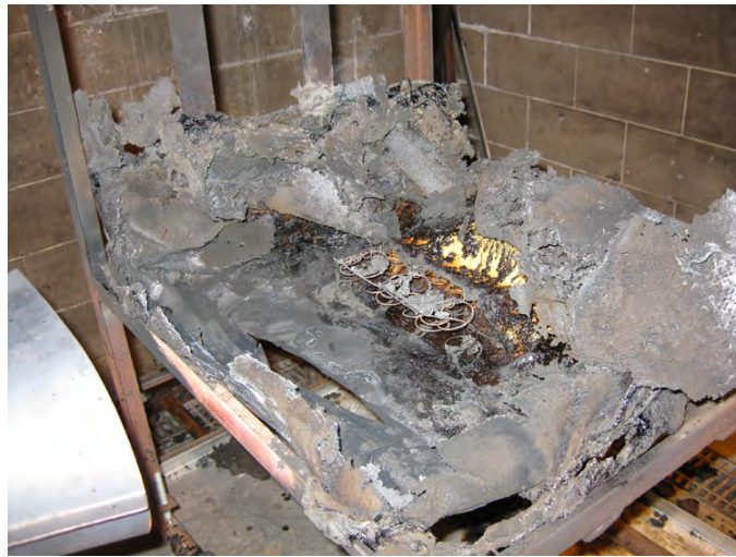
Figure B-15. Close-Up View of Baseline Test 1 Cushion Following Laboratory-Scale Test (typical)
