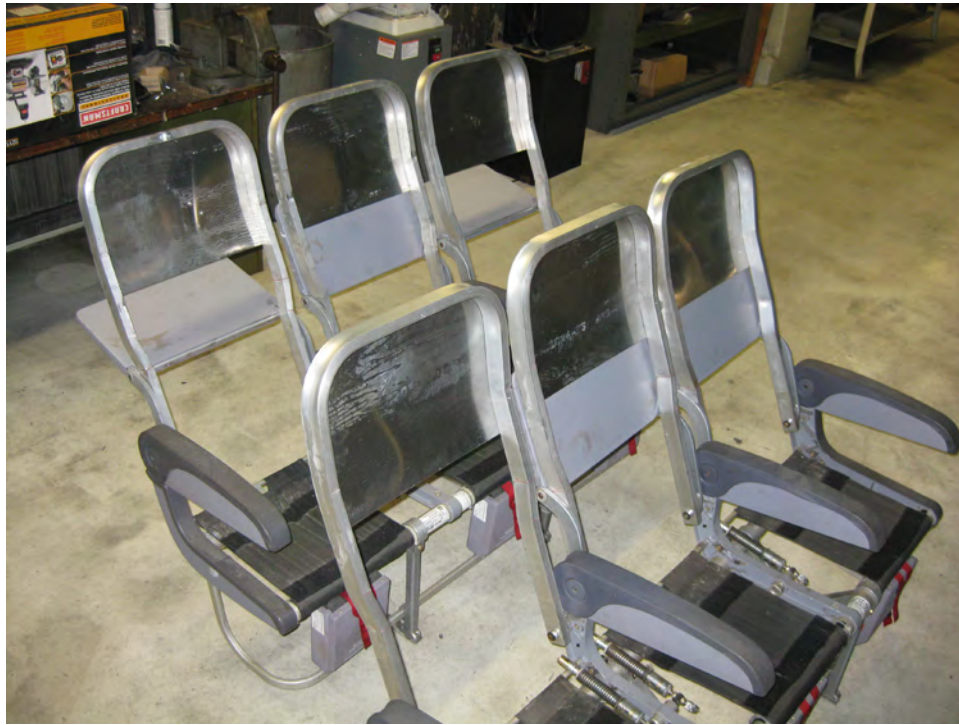
Figure A-6. Fabrication of Seat Assemblies Using Alternate Seatbacks
