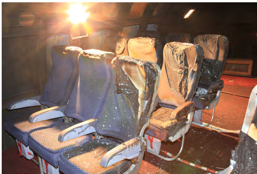
Figure 102. Starboard-Side Seats Showing Minimal Damage
