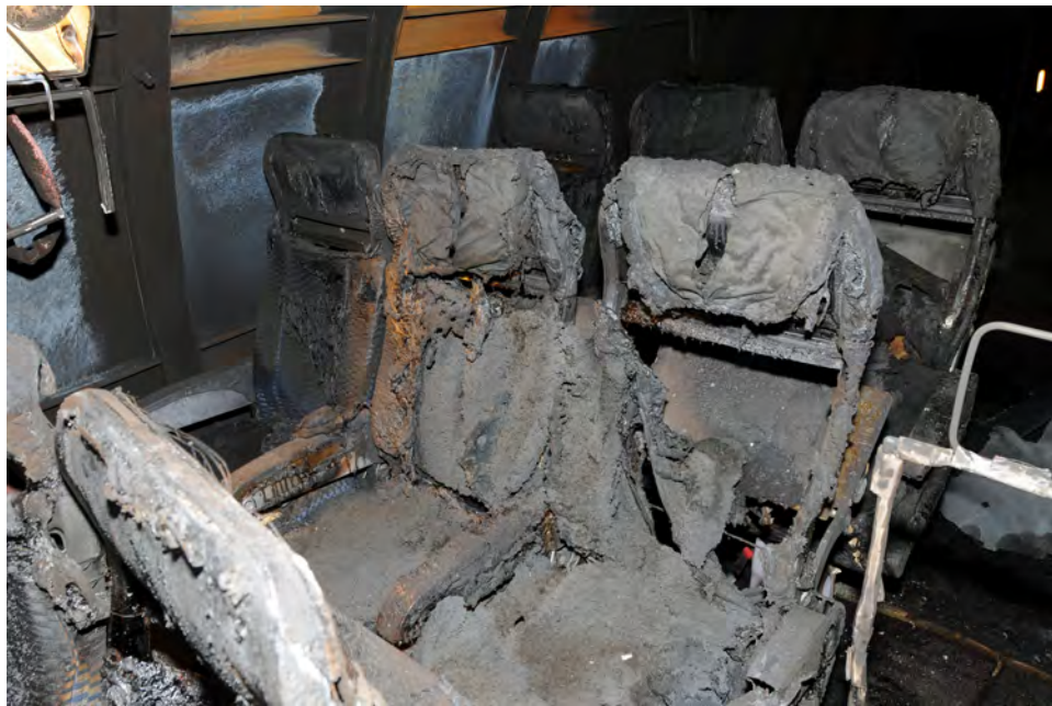
Figure 62. Close-Up View of Starboard-Side Triple Seat in the Baseline 2 Test
