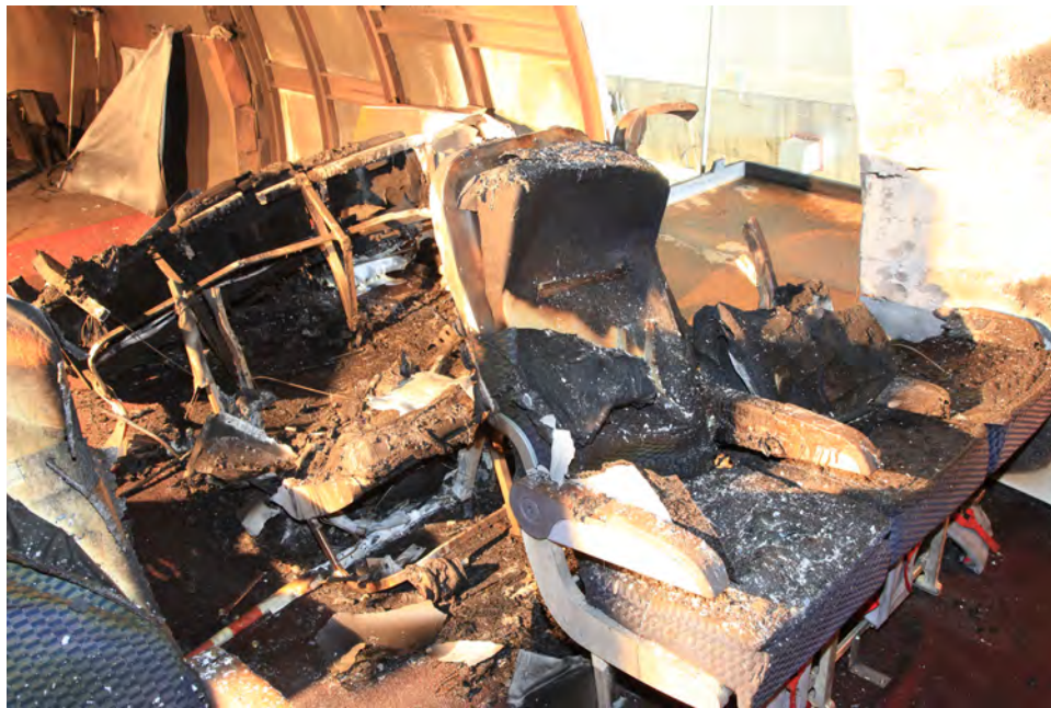
Figure 100. The WE-43 Magnesium Alloy Posttest Results
