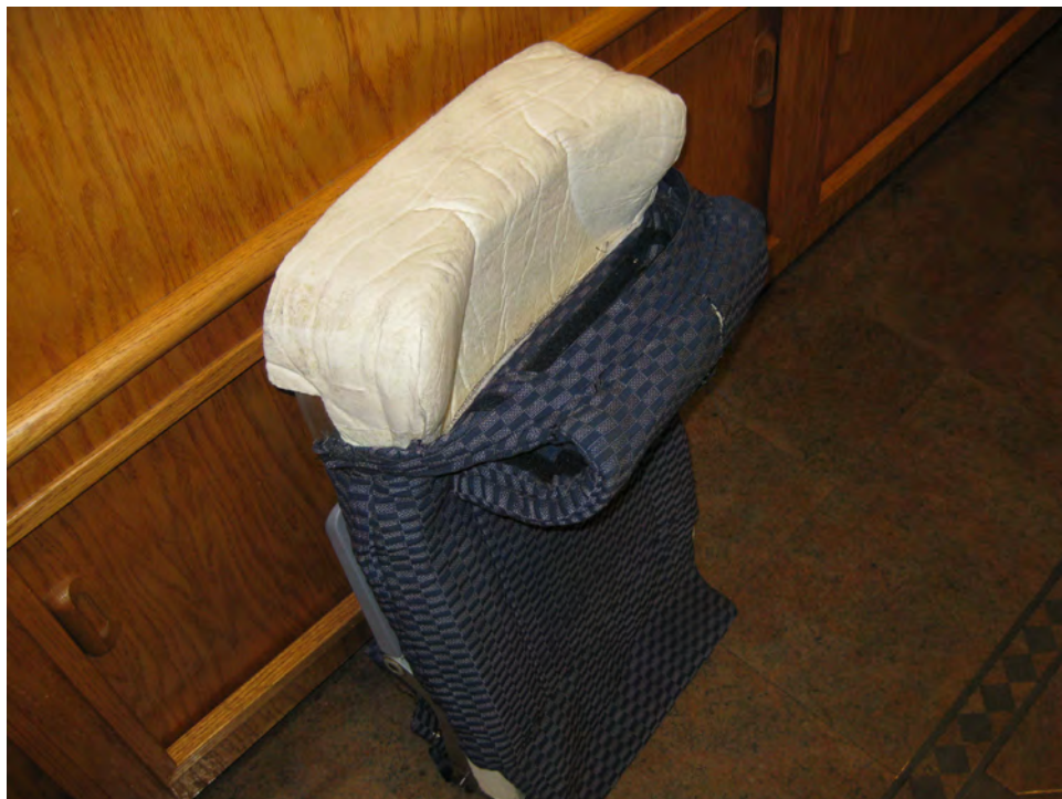
Figure A-5. Front View of Dress Cover Used in Alternate Seatback Assembly
